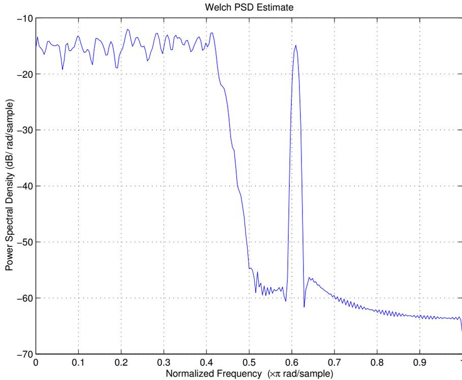
From the spectrogram, it looks like there is a tone that goes up and down and up and down with a lot of noise underneath that signal. The rising and falling tone goes between the frequencies of around 6kHz to 8kHz. The noise is spread-spectrum between 0Hz and around 5kHz, which can be seen from on the graph of power spectral density.
