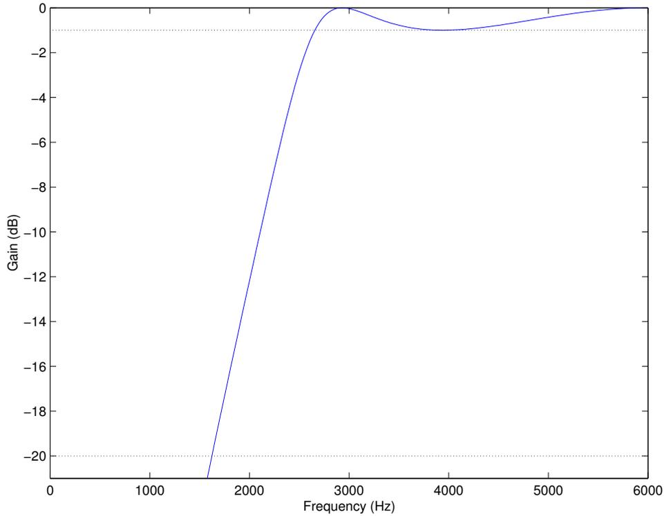
4. As you can see from the plot above, the given filter has no more than 1dB attenuation in the passband (above 3kHz) and that the filter also passes through the 20dB attenuation mark at the beginning of the stopband (1.6kHz). This means that the digital filter is within the specification given.
