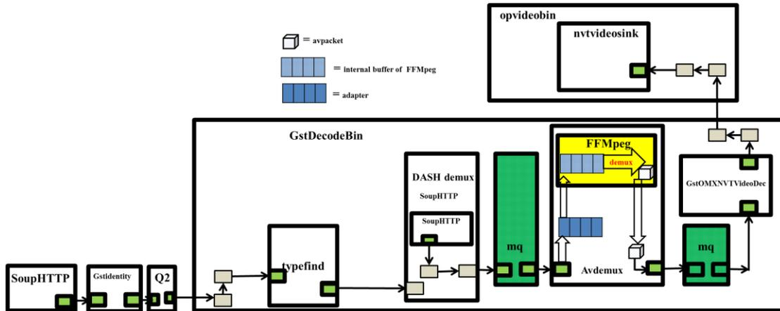
Settings of OK's internal buffer (mq0 & mq1 in green)
