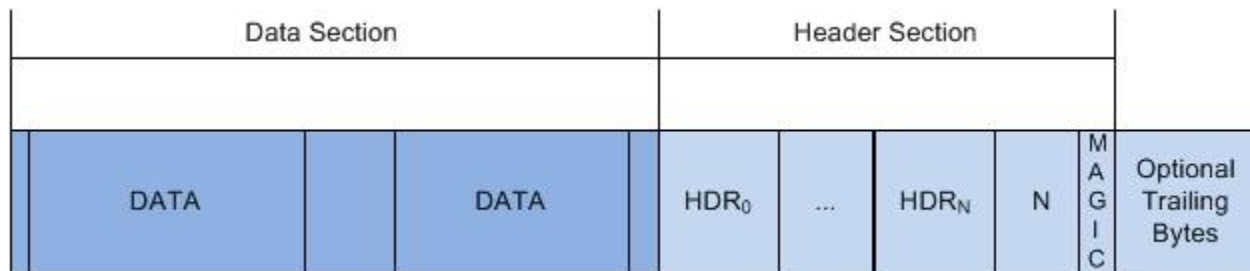
Illustration 2: Skype Transport Stream Packet
